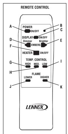
When using the remote control, the power on/off switch inside the body and the wall switch (optional kit) must be on the OFF position.
